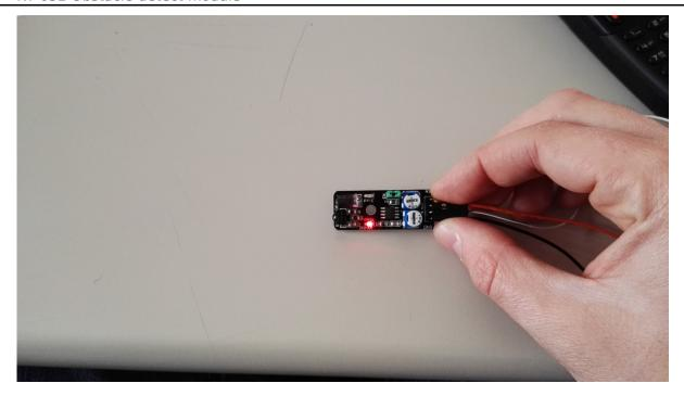
Condition 2: Detector detects an obstacle [LED on the module: ON] [Sensor Signal= Digital Off]
