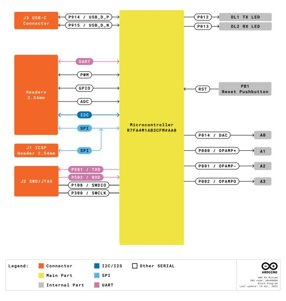
Arduino R4 Minima Block Diagram
